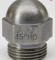
The HO series is offered to meet the requirement for Nozzles to be used on higher viscosity oils at elevated operating pressures. It is a redesignation of the PLO-HO, PL-HO and R-HO series to simplify specifications for ordering. These Nozzles (as with all Monarch Nozzles) are stamped with their nominal flow rate at 100 PSIG on #2 fuel oil and are available in capacity sizes from 1.00 through 100.0 GPH.
