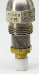
The BPS nozzles produce variable orifice flow rates by by-passing fluid from the nozzle swirl chamber. The orifice flow is regulated by controlling the by-pass line pressure.
